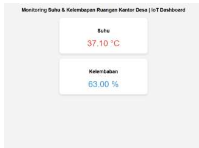
Gambar 4. Dashboard monitoring suhu dan kelembapan secara real-time
