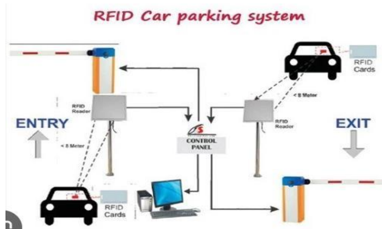
Gambar 6. RFID Car Parking system
