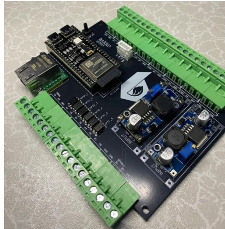
Gambar 5. Sistem hardware smart greenhouse berbasis ESP32
