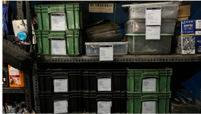
Figure 3. Fast-Moving Spare-Part Storage Boxes After Label Installation at KMR
